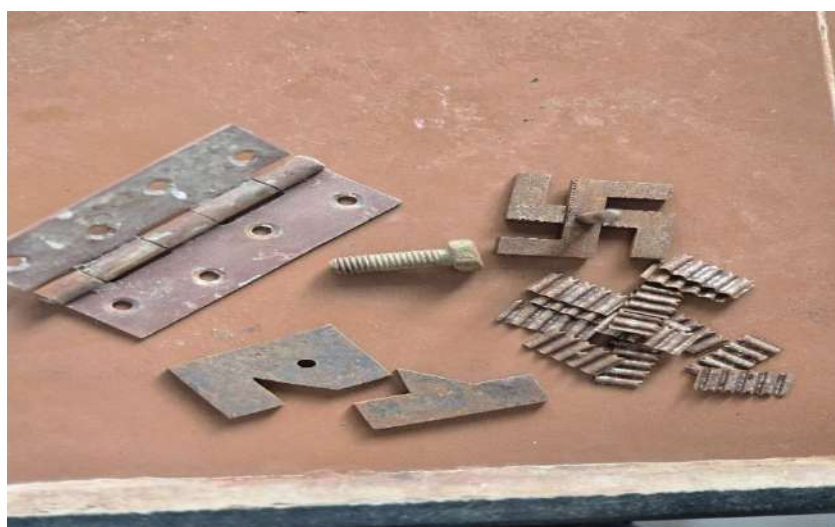
Figure 3.2: Corroded Iron Particles Used for Pickling
