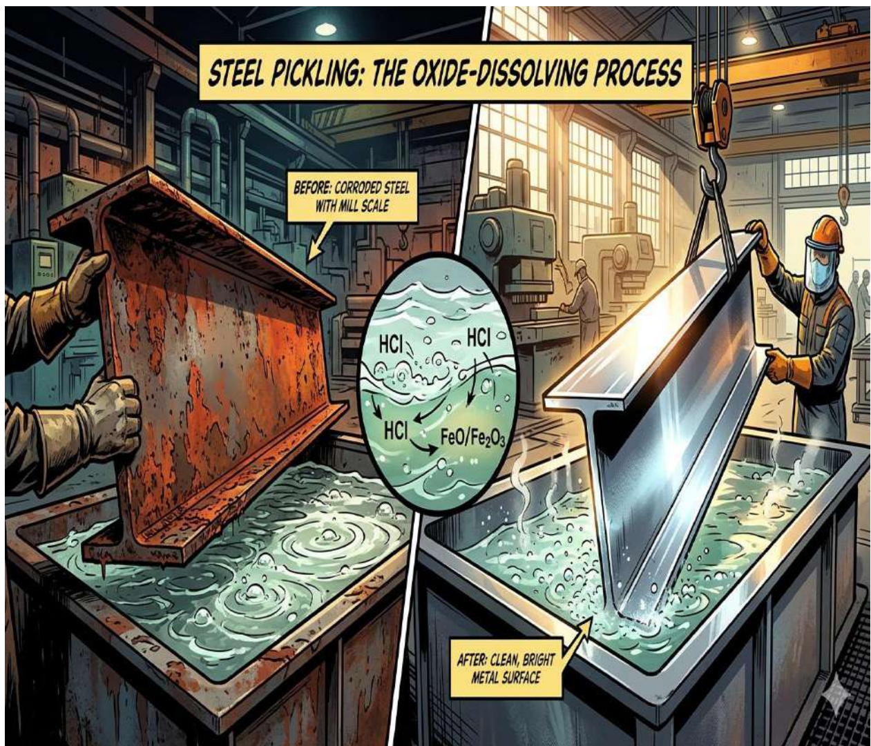
Figure 1.1: Steel Pickling Process Showing Removal of Oxide Layer
