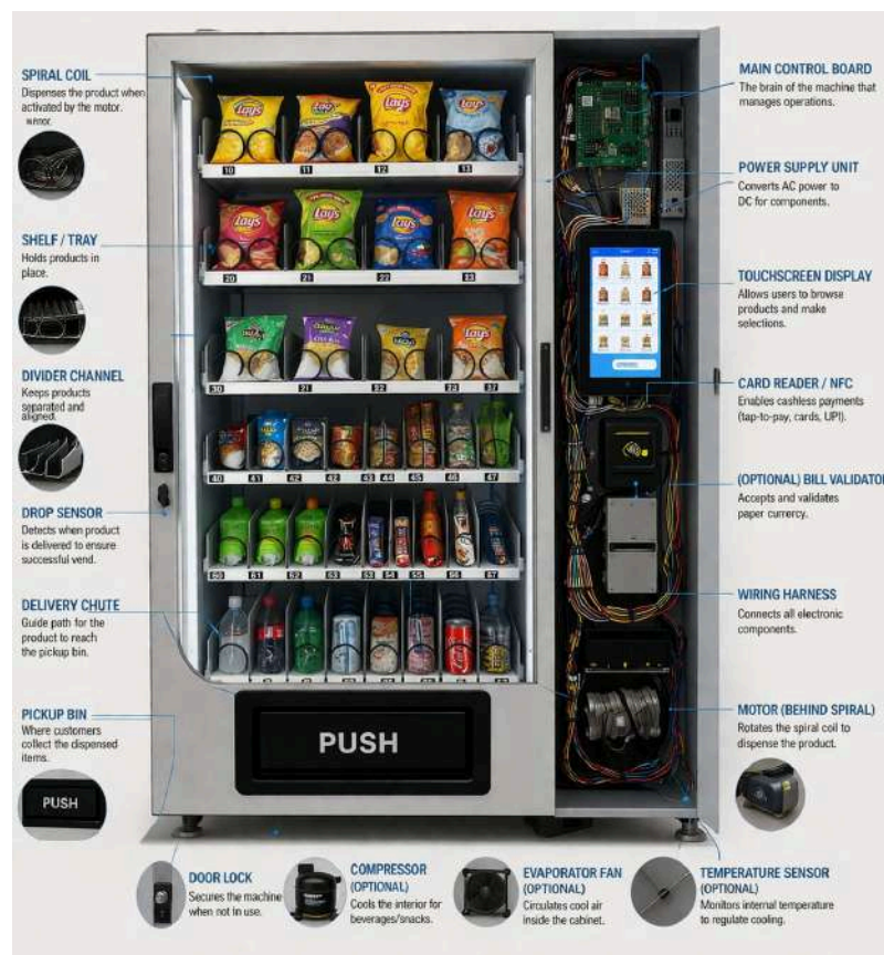
Fig 2: Snack Vending Machine Internal Components — Coil Motors and Slots
